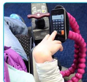
One device to help with switch positioning is Flexzi.
